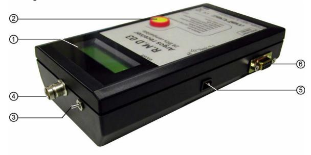
Receiver, processor and battery are protected by a hand-held housing, dimensions  $195 \times 100 \times 44$  mm. The top panel includes a  $2 \times 16$ -character LCD screen (1) and a pushbutton (2). This pushbutton is used to start the receiver and to access to various functions.
