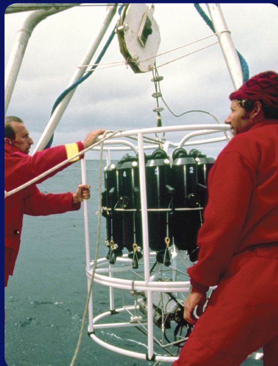
Full-size, 12-bottle SBE 32 Carousel Water Sampler with Extension Stand for CTD
