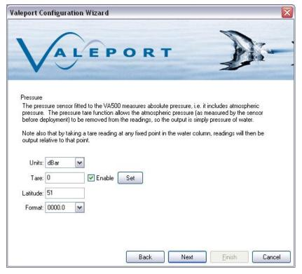
If the Altimeter is fitted with the optional pressure sensor, this can be configured here.
